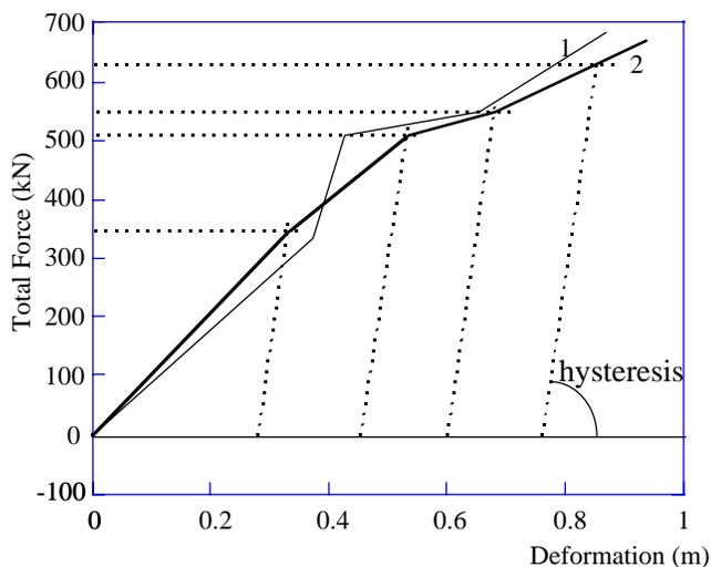
Figure 6a. Comparison between real-time approximation (curve 1) and post-crash data, based on measurement of hysteresis (curve 2)
