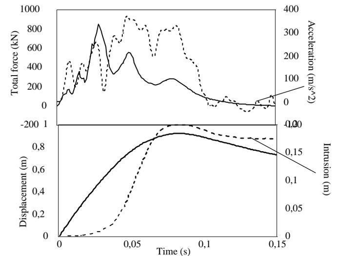
Figure 4b. Time-histories of barrier force, vehicle acceleration, deformation and intrusion in the full frontal high-speed test.
