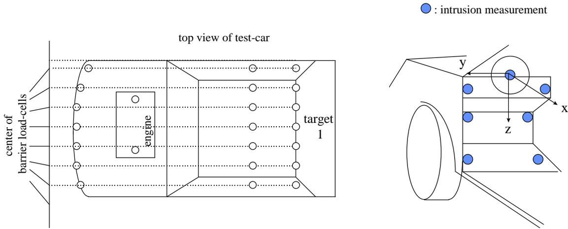
Figure 2. Location of the targets for displacement and intrusion measurements.
