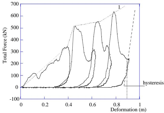
Figure 5. F-D curves of the full frontal repeated crash tests, with curve 1 ( . . . . ) an estimated of the stiffness.
