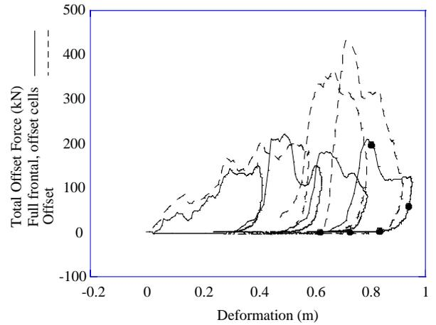
Figure 10. F-D curves of the total force in offset repeated tests vs. that of the total force of 18 corresponding load-cells in full frontal repeated tests.
