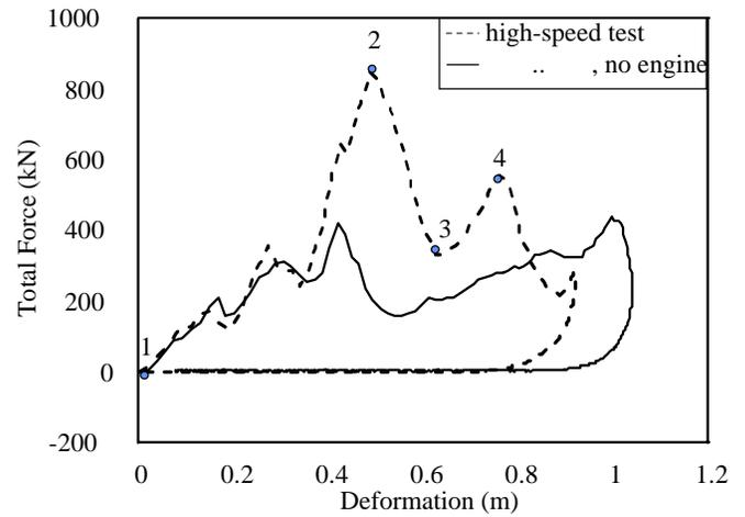
Figure 7c. Comparison of the F-D curves in the high-speed full frontal tests with and without power-train. 1)  $t=0.0$  s, 2)  $t=0.028$  s, 3)  $t=0.038$  s, 4)  $t=0.05$  s
