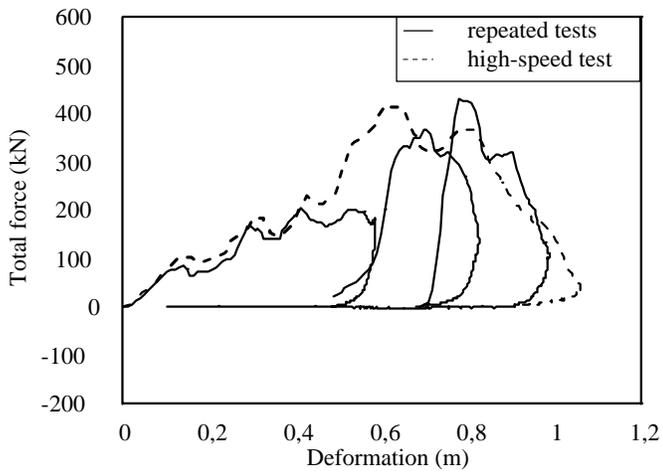
Figure 7b. Comparison of the F-D curves in 50% offset high-speed and repeated tests
