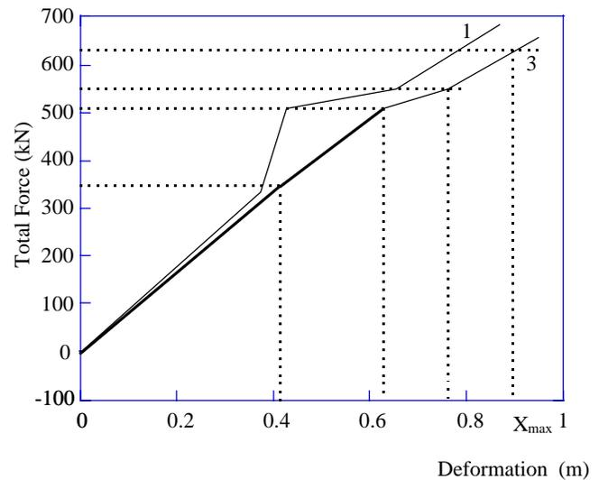
Figure 6b. Comparison between real-time approximation (curve 1) and post-crash data, based on measurement of maximum crush (curve 3)
