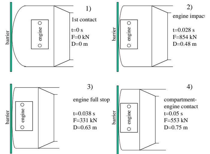
Figure 4a. Top-view of the car in a high-speed in full frontal test at  $t=0$ ,  $t=0.028$ ,  $t=0.038$  and  $t=0.05$ . The corresponding barrier force and vehicle deformation are included.
