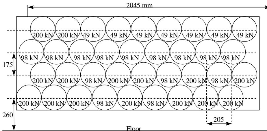
Figure 3. The load-cell barrier with the force range per cell
