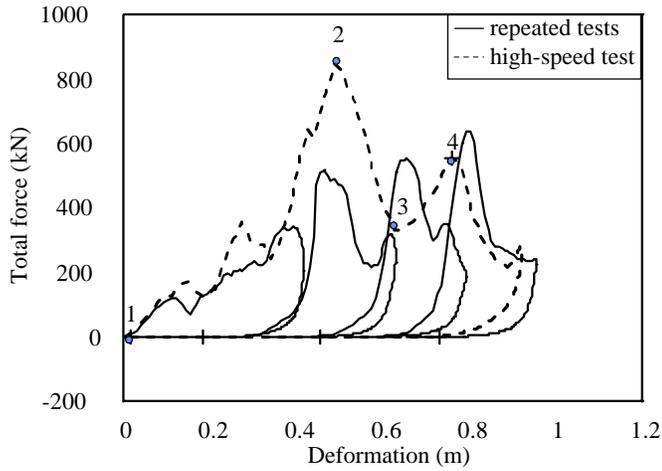
Figure 7a. Comparison of the F-D curves in the high-speed full frontal test with repeated full frontal tests. 1)  $t=0.0$  s, 2)  $t=0.028$  s, 3)  $t=0.038$  s, 4)  $t=0.05$  s
