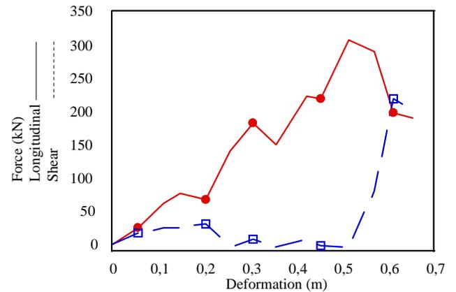
Figure 11. Shear and compression stiffness with deformation
