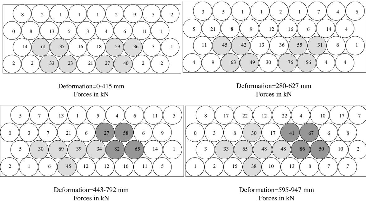
Figure 8. Maps of load-cells with local forces (kN) in each test repetition
